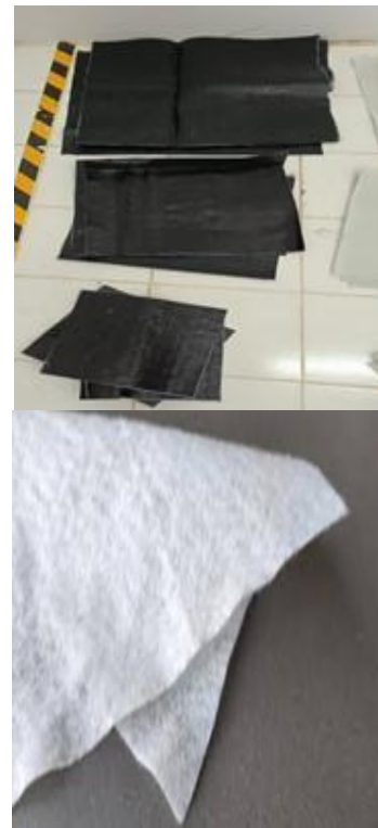
Figure 1: The types of Woven and Non-Woven Geotextiles
