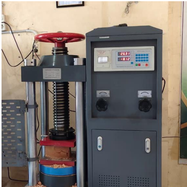
Figure 3.7. Compressive Strength Test Equipment
