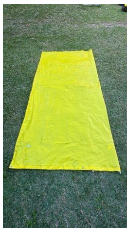
Figure 2 – Soil isolation with plastic sheeting.
