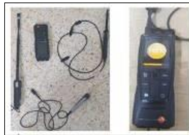
Fig. 10. Measurement instruments: Testo 480-AG 5011ST
